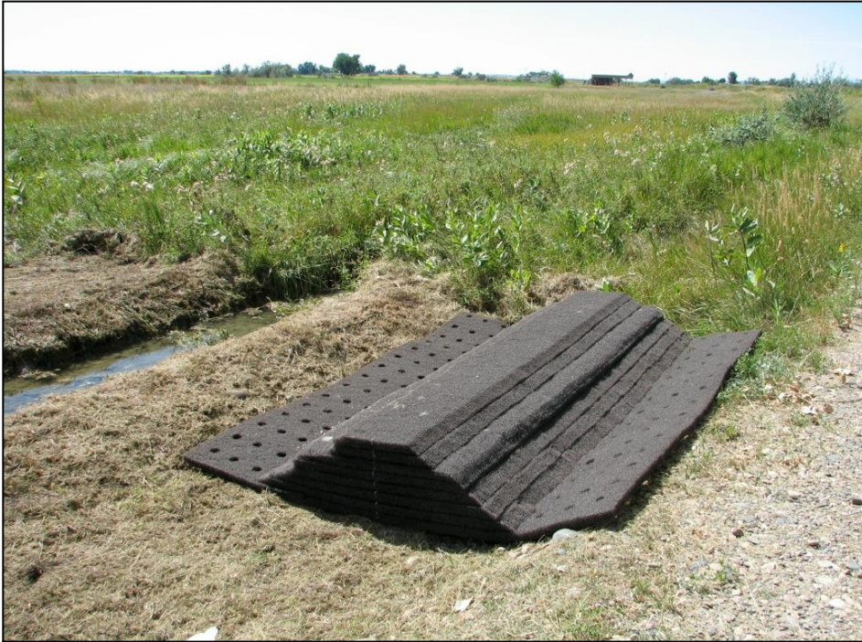
Figure 2. Inverted bioswale before installation
