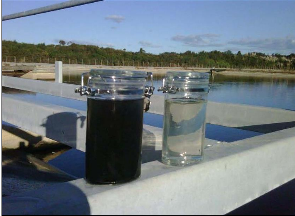
FTW influent (left) vs. effluent (right) at McLean's Pit, May 2010
