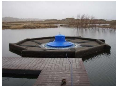
**Figure 4.** Pump mounted in floating island
