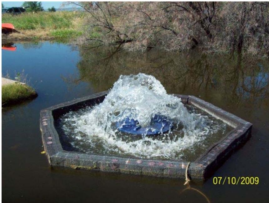
**Figure 8**– Prototype Island #2 with 1.5-hp aeration/circulation pump
