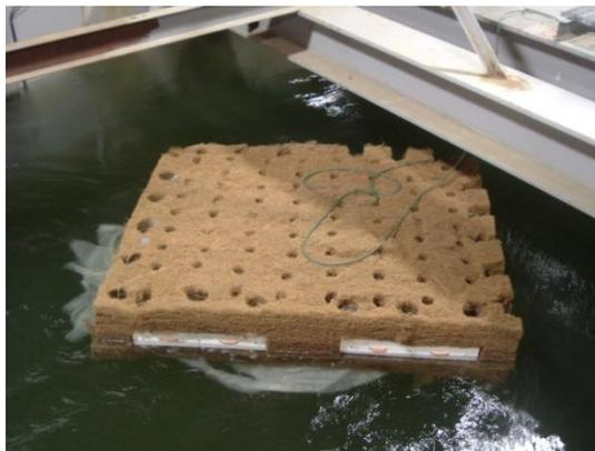
BioHaven® module in current testing flume
