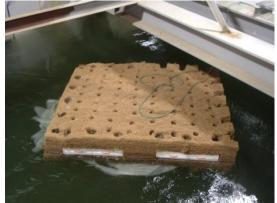
BioHaven<sup>®</sup> module in current testing flume
