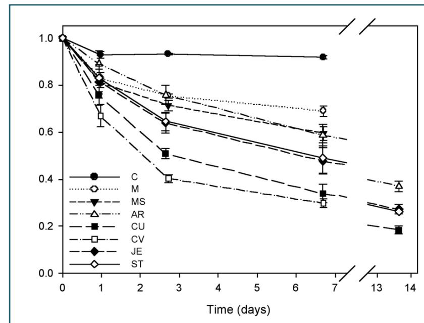
Figure 5 – Mean proportion of Total Cu concentration remaining (C/Cin) for each treatment (n=6). Initial concentrations (Cin) ranged from 0.010 to 0.01 gm<sup>-3</sup>. Note that 14 day samples were only collected for some treatments (AR, CU, JE and ST) during one batch (n=3)
