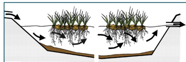
Figure 1 - Schematic longitudinal cross-section through a typical Floating Treatment Wetland system. Note that the water depth can vary appreciably in such a system without affecting plant growth. (Source: Headley and Tanner, 2006)
