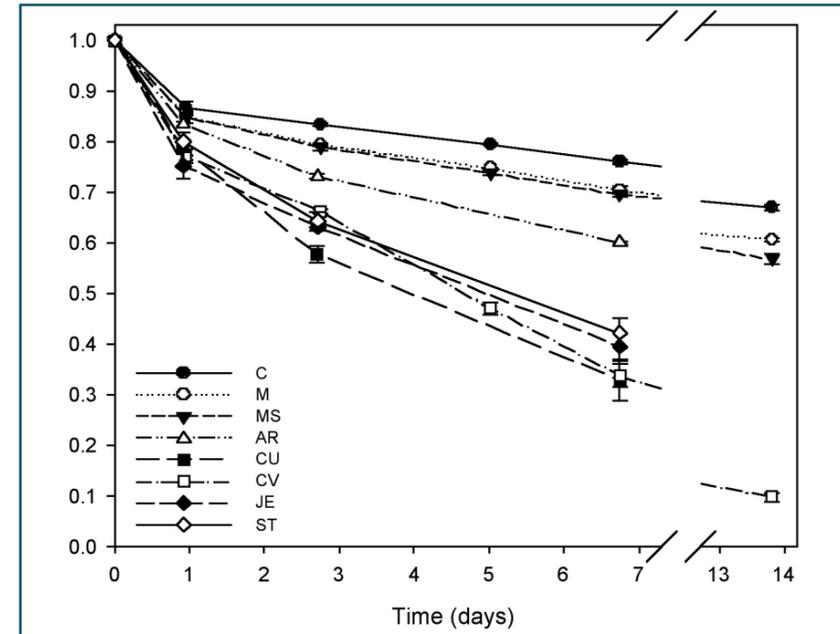
Figure 4 – Mean proportion of Turbidity remaining (C/Cin) at 20cm from the bottom of the tanks for each treatment (n=3). Initial concentrations (Cin) were 10.2NTU. Error bars (not always visible) represent ± one standard error of the mean. Note that 14 day samples were only collected for some treatments (AR, CU, JE and ST) during one batch
