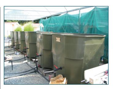
Figure 2 – Six of the 12 mesocosm tanks used in the batch experiments
